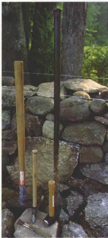
Tools are simple. A basic tool kit includes an 8-lb. sledgehammer, a 3-lb. sledge, a stone hammer, a chisel and a pry bar.
